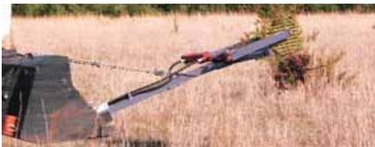
Expanded metal grips can be used to grab brush or pull small trees out of the ground.
