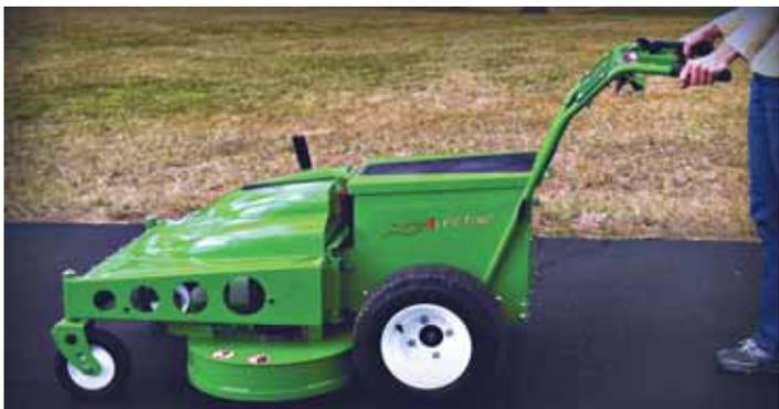
Mean Green mower uses commercial-grade wet-cell, lead acid batteries that hold their charge longer than typical deep cycle batteries.
