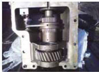
Modified transfer case has a detent spring on the fork shaft, allowing Weaver to slip into 4-WD on-the-go.
