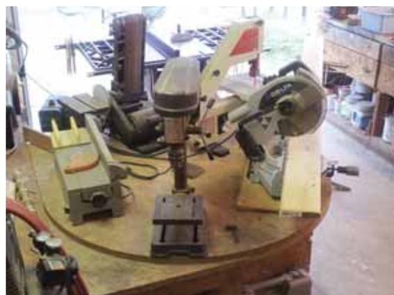
A 48-in. dia. rotating tool table provides David Chambers with easy access to a cut-off saw, drill press, band saw, planer and combination belt/disc sander.
