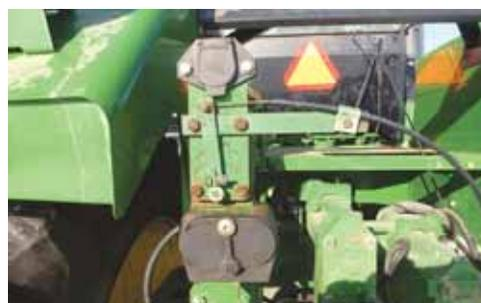
Simple lever and cable device lets Murry McMillan adjust the hydraulic flow control valve on his tractor without leaving the driver's seat.
