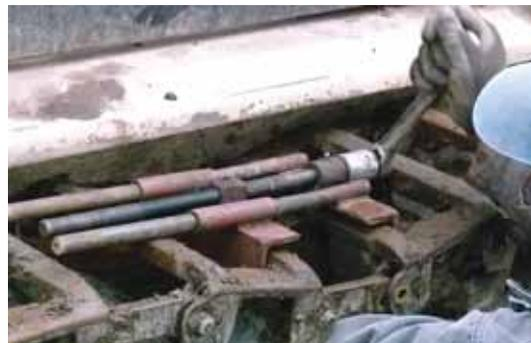
Track tightener for skid loaders uses a threaded bolt to draw the loose ends of the tracks together, making it infinitely adjustable.
