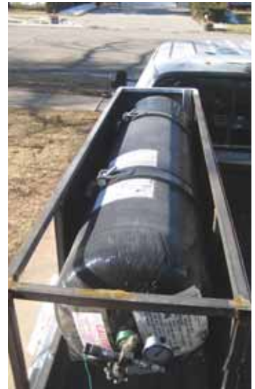
Kits for pickups replace 50 to 75 percent of the diesel fuel in each piston stroke with compressed natural gas (CNG).
