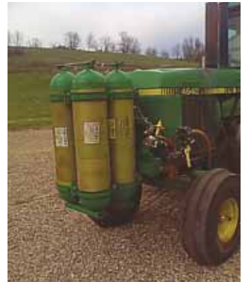
Ed Jones mounted CNG canisters on front of his Deere 4640 tractor. He says burning CNG boosts horsepower by 30 percent.
