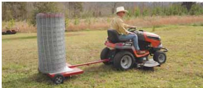
2-wheeled “fencing trailer” consists of a metal platform with a 34-in. long pole on top and a poly foot plate for the wire roll to turn on.
