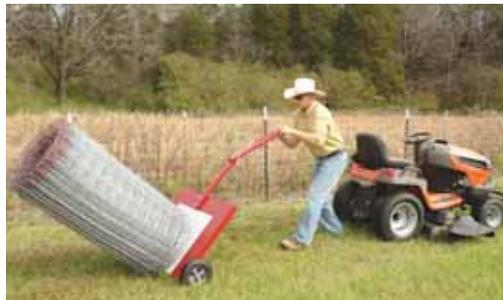
To load the wire roll, you grab a pair of handles at one end of tongue and pull it back toward the ground until the roll is in a vertical position.
