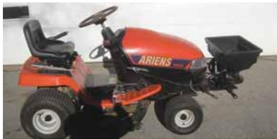
Jerry Bruecker removed the wheels, tongue and gearbox from a pull-type spreader and mounted it on front of his garden tractor.
