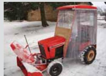
refrigeration supply store. The strips came with pre-punched holes at one end and were 8 in. wide and 8 ft. long when Borden bought them. He cut each strip to length and overlapped the strips 4 in. He used 1/4-in. bolts to attach the strips to a metal strap -- purchased ready-made from the manufacturer -- that's bolted to both sides of the cab roof.
