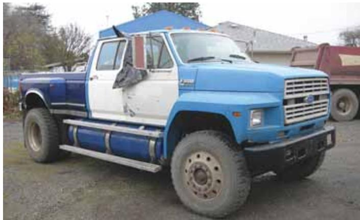
Doug Fry converted his 1987 Ford F-800 into this 210 hp dually pickup equipped with a crew cab. It's fitted with twin 115-gal. fuel tanks.
