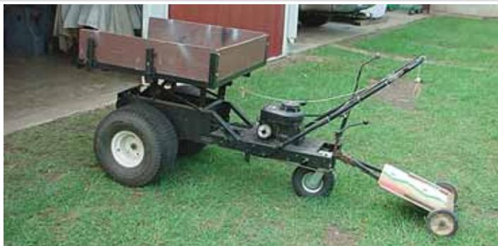
Ron Forster's home-built self-propelled cart is powered by a 3 hp engine and 5-speed transmission. The operator stands on a 2-wheeled plywood platform.
