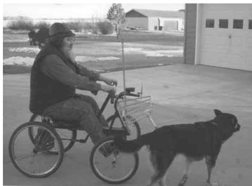
Split axle cart is fitted with a homemade "eccentric" drive on one side that's powered by pumping on a T-handle. A big dog can also be used to pull the cart.
