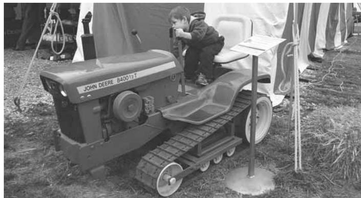
Ervin Schulze built this "mini" Deere 8400 tracked tractor by converting a Deere 140 garden tractor. "It looks realistic and drives like the real thing," he says.
