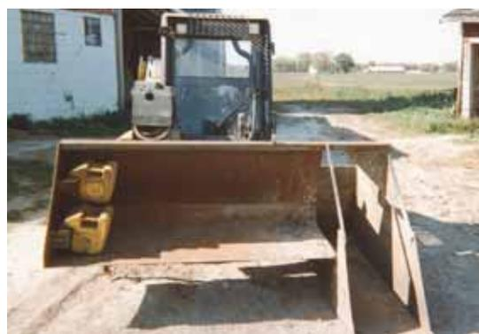
An 18-in. wide "chute" extends 1 ft. below bottom of bucket and into gutter. As operator drives forward, manure slides into the chute over into bucket.
