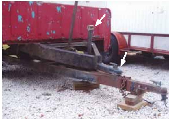
Wallace Goldman modified this 2-wheel trailer so he can dump it with an ordinary bumper jack. Arrows point to jack and ball hitch lock-down.
