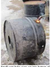
Small vent holes were cut into bottom of barrel, with a larger hole at the top for smoke to exit.
