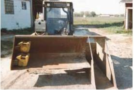
An 18-in. wide "chute" extends 1 ft. below bottom of bucket and into gutter. As operator drives forward, manure slides into the chute over into bucket.
