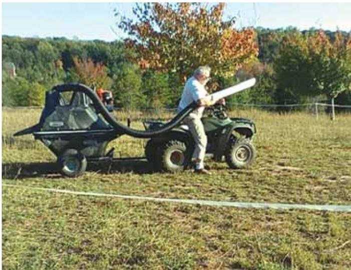
Sam McNair's homemade, tow-behind vacuum turns horse manure into a fluffy, dry material that's ready to compost.
