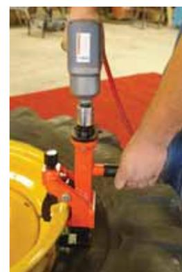
All you need to operate impact bead breaker is a 1/2-in. drive impact wrench. Handle on back of tool is used to apply leverage as you draw tire in.
