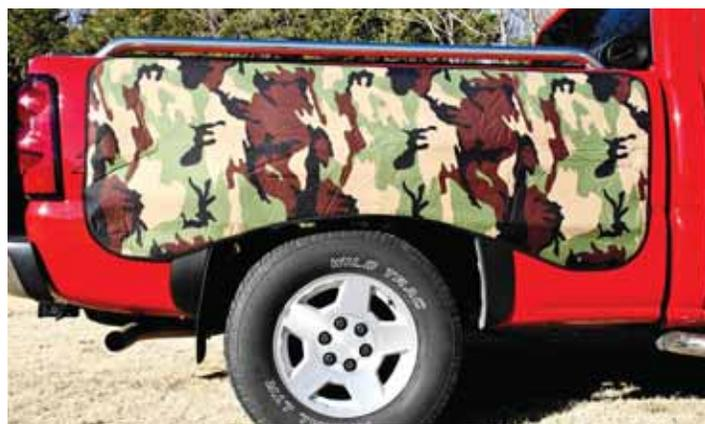
Truck Chaps are made from Cordura nylon with a foam layer in the middle. They're held in place with 8 small rare earth magnets.
