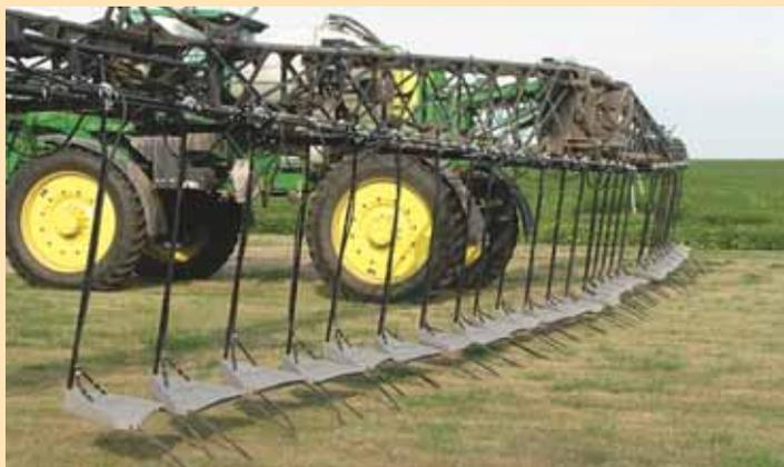
**Vertical drop bars fasten onto sprayer toolbar, with a plastic Y-shaped piece attached to the bottom. A pair of drag hoses deliver product within 2 to 3 in. of the row.**
