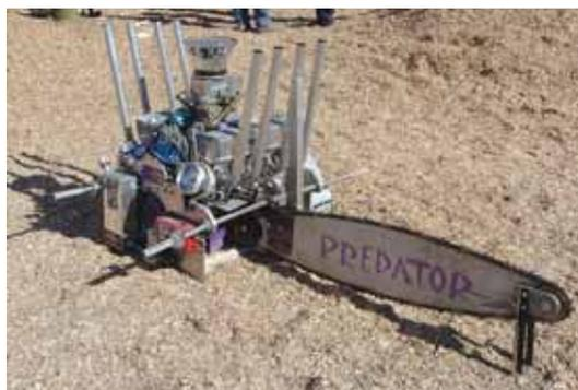
**Giant Predator chainsaw is powered by a Buick V-8 engine with 300-plus hp. It once cut through a 30-in. log in .088 seconds.**
