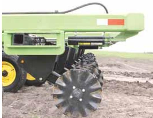
**Independent gangs of wavy coulters are each controlled by a hydraulic cylinder, allowing operator to change coulters penetration angle up to 9 degrees.**
