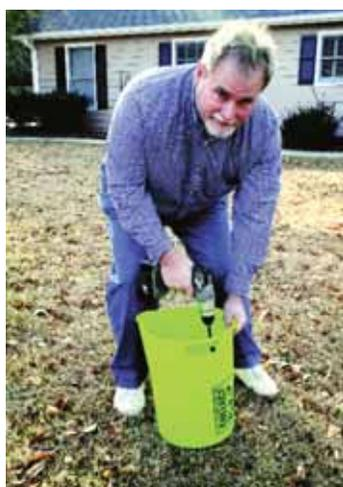
Collector tube extends up from bottom of bucket. To collect soil sample, the operator runs a cordless drill-powered auger through tube and into the ground.
