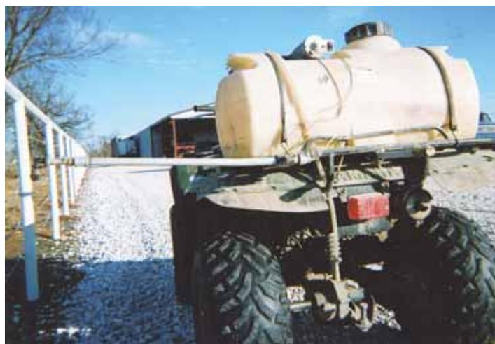
Fence row sprayer is made from a 3-ft. long galvanized pipe with a flexible nipple and spray nozzle at one end. Nipple bends and won't break if it hits fence.
