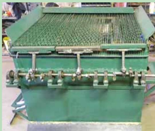
Cranks at end of machine raise and lower sections of serrated teeth that move between flat steel bars. You can see a video of it in action at the company's website.
