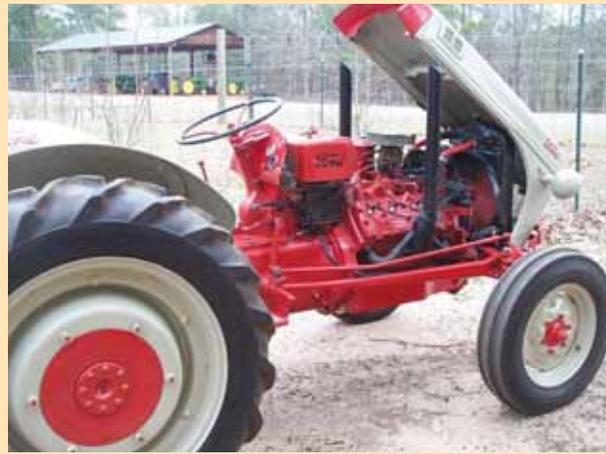
Ernest Godbee repowered his Ford 9N tractor with a Flathead V-8, lengthening the hood to allow for the longer engine.
