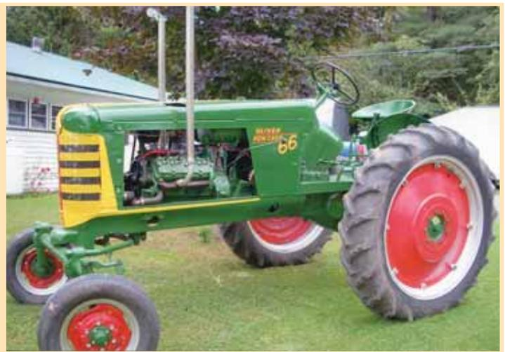
Lloyd Stetson's Oliver 66 "purrs like a kitten" after he repowered it with a 1938 Ford Flathead V-8.
