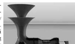
**Inverted cones funnel wind down into underground turbine.**
