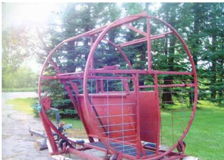
Rolling squeeze chute is made from a wire spool, with a trimming chute at the center. A winch is used to rotate the chute.
