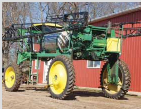
Articulated steering lets sprayer’s rear wheels exactly track the front wheels on end rows. When desired, the articulation joint locks and front-wheel steering takes over.
