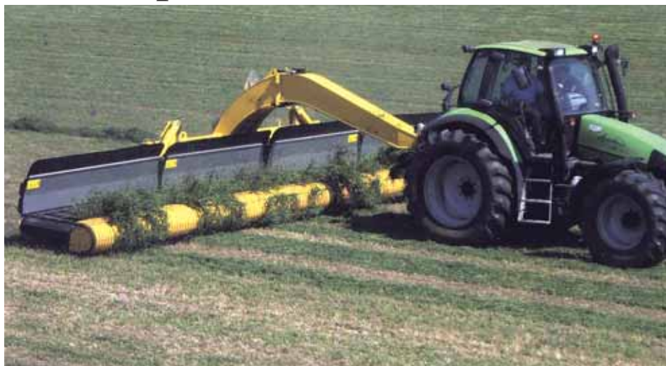
Merger's suspension system controls ground pressure and oscillation of pickup heads as well as transport wheels.
