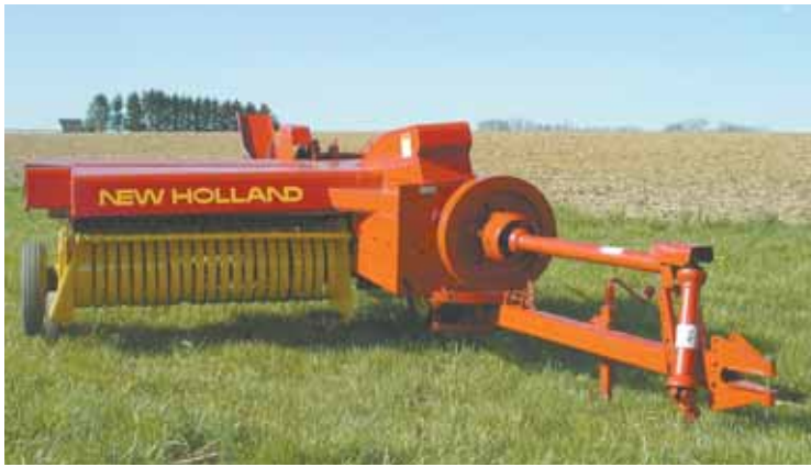
Completely reconditioned NH baler makes 8 by 11-in. bales with variable length from 16 to 24 in.
