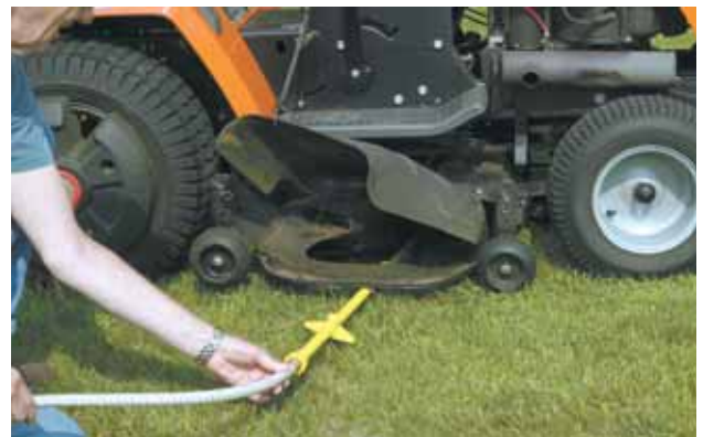
To clean the deck, you connect the washer to a garden hose and slide it all the way under the deck. Then you turn on the water and also turn on the mower.
