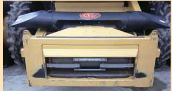
EZ-View Dust Diverter can be installed in 30 min. or less and the ends flip up for easy cleaning.
