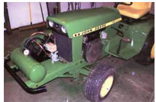
An old electric air compressor and a small portable air tank mounts on front of Sands' Deere garden tractor. Compressor is belt-driven off tractor engine.
