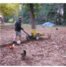
Worker Bee, an electric-powered, walkbehind tractor, is designed to do many different kinds of jobs.
