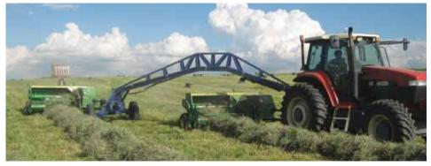
Dale and Richard Hallett built this double hitch for their small square balers. Connecting arch contains no gearboxes or driveshafts, only hydraulic hoses.
