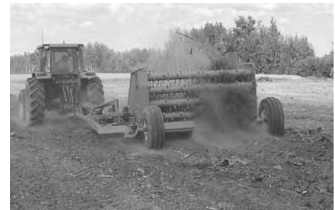
Home-built "root piler" moves everything from 2-in. dia. roots to 12-in. dia. logs up to 8 ft. long. It makes an 8-ft. wide swath.
