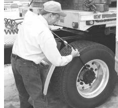
Tire Bee repair kit uses a selfvulcanizing plug and a tool that uses compound leverage to push plug all the way through the tire. One end of tool is secured on wheel rim.
