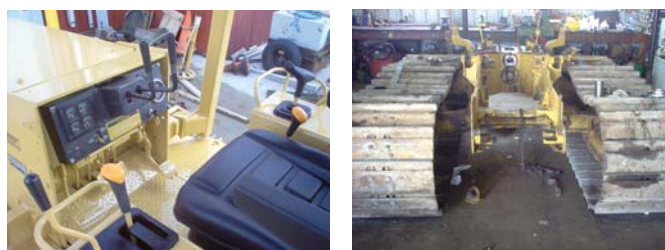
A new H-pattern steel housing and linkage was fabricated for the Deere transmission and mounted next to the seat (above left). Ammon started out by stripping the engine and 3-speed transmission off the Cat's chassis. Tractor is powered by a 6-cyl., 6.8-liter Deere Power Tech engine.
