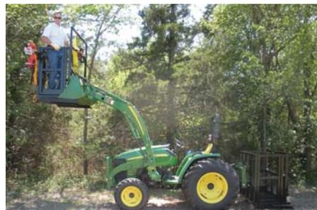
"Bucket basket" straps into front-end loader bucket to provide a safe work platform. It can hold 1 or 2 people.
