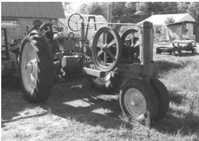
Orville Schraeder mounted a stationary Witte engine on his Deere B tractor. Homemade flywheel pulley replaces tractor's flywheel.
