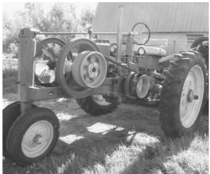
A reverse belt drive connects engine-mounted pulley to pulley on tractor's flywheel.
