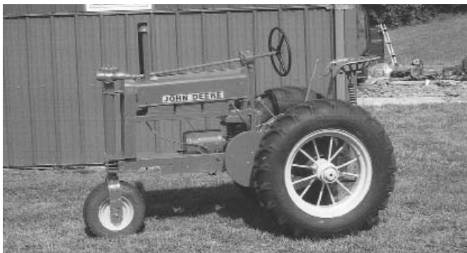
Half-size 1938 Deere A is powered by three 12-volt deep charge batteries. But thanks to an on-board recording, the mini tractor sounds like a full-sized Deere.
