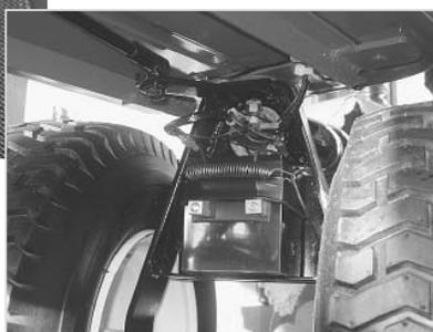
Underside of wagon shows articulated steering system.
