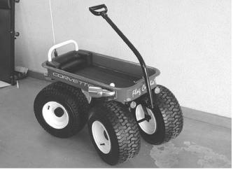
Radio Flyer wagon rides on big garden tractor tires and has a padded vinyl seat and rollbar on back. Note side-by-side Corvette C-5 exhaust mufflers.
