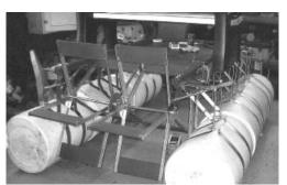
Paddleboat's platform is connected to drums by a metal framework.
