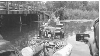
Home-built pedal boat floats on eight 30-gal. plastic drums, and is fitted with a wood and plastic seat set on a plywood floor.
