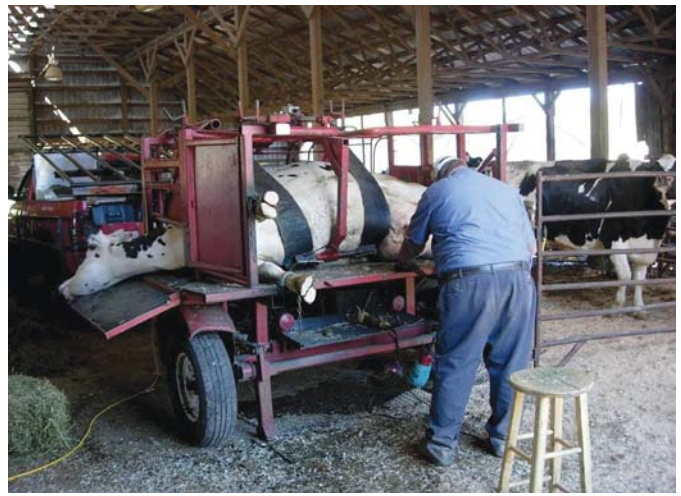
Unit is fitted with dual hydraulic pumps, which causes the tilt table to go up and down fast.
