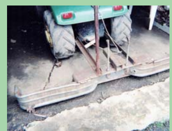
Russell Burdett made a blade to level his driveway out of scrap parts and an old Chevy pickup bumper.
