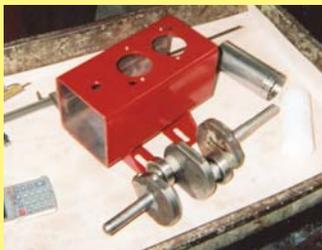
Pressurized air powers the pistons and crankshaft.
