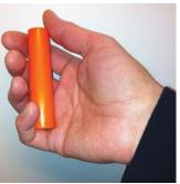
Bolus is inserted down cow's throat into stomach. It sends cow's temperature to a software program each time the animal walks through a reader panel.
