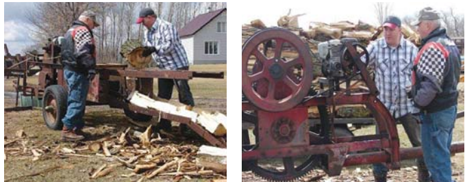
Operator drops a chunk of wood into the bale chamber, and pieces come out bale chute (left). Baler's flywheel transfers power to plunger, which pushes wood into wedge.
