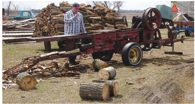
Mike Paquin fitted his New Holland baler with a 5 hp Honda engine, cut a hole in the top of the bale chamber, and welded a splitting wedge in place at the end of chamber.
