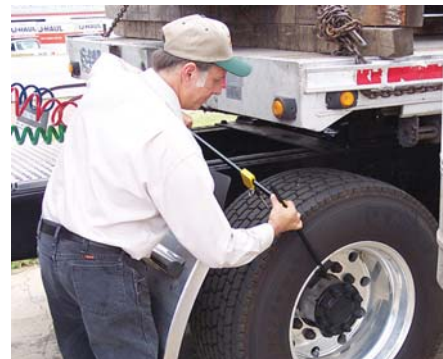
Tire Bee repair kit uses a self-vulcanizing plug and a tool that uses compound leverage to push plug all the way through the tire. One end of tool is secured on wheel rim (lower).
