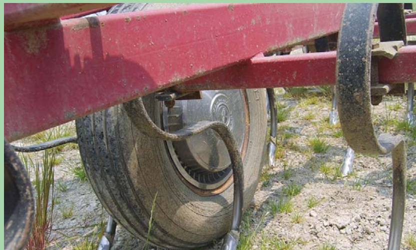
To protect the valve stems on his field cultivator from trash, Joe Thompson snapped hub caps off an old pickup onto the cultivator's wheels.
