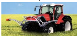
Isaria crop reader mounts on front of tractor to map fields and determine crop needs.
