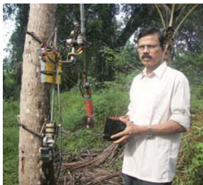
Coconut-harvesting robot is controlled by a hand-held remote from up to 100 ft. away.
