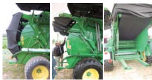
Canvas clamshell rear gate opens quickly to eject bale. Inside there are just two large rubber belts.
