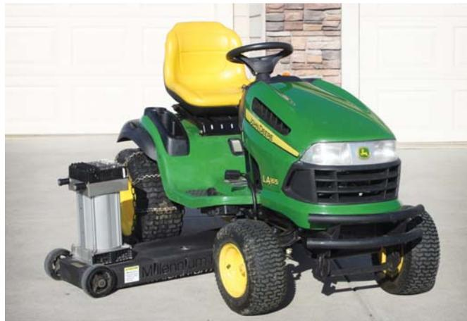
To use you slide the mower deck out and slide generator into place, then slip on the belt and tension with a ratchet strap.
