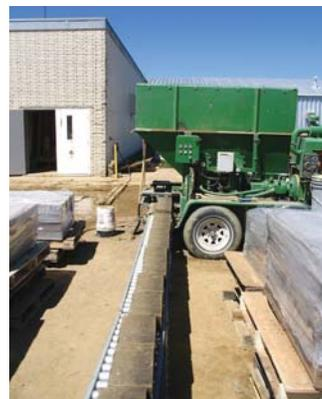
Earth bricks can be left exposed like a fired-brick wall (left). Earth block buildings are produced on site with local soils.
