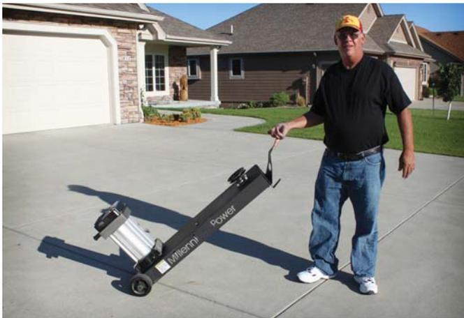
Generator rolls like a 2-wheel cart and is powered by the engine on any riding lawn mower or garden tractor.
