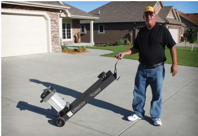
**Generator rolls like a 2-wheel cart and is powered by the engine on any riding lawn mower or garden tractor.**
