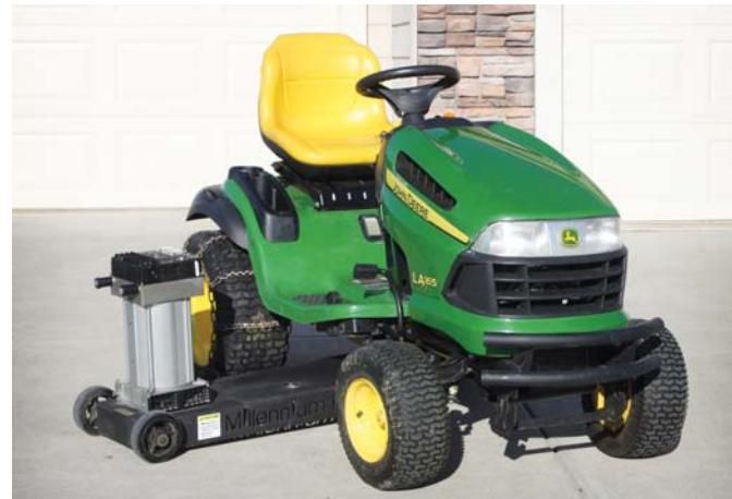
**To use you slide the mower deck out and slide generator into place, then slip on the belt and tension with a ratchet strap.**
