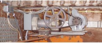
Door is raised and lowered by an electric hoist that was originally used to lift basketball hoops out of the way inside a gym.
