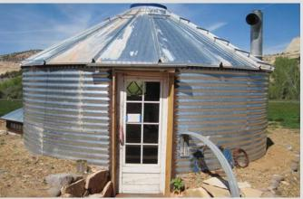
Scott Brodie built this 2-floor combination root cellar-storage shed out of an 18-ft. dia. corrugated steel bin, installing a white entrance door on front.
