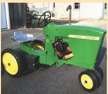
Tom Demers motorized this 1965 Deere Pedal Trac by installing an Echo 21 cc weed trimmer engine. It hooks up to a transmission off a Troy-Bilt mini rototiller, which chain-drives tractor's rear axle. Photo at left shows underside of tractor.
