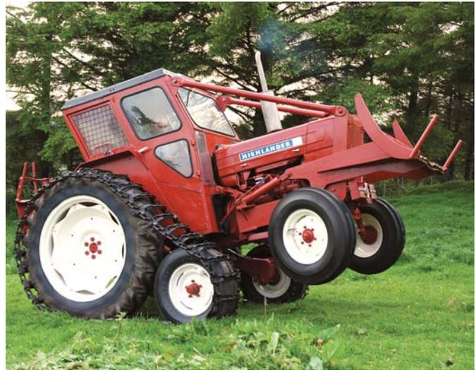
Lowering the idler wheels with a hydraulic ram raises the front end off the ground, preventing the front wheels from sinking in.
