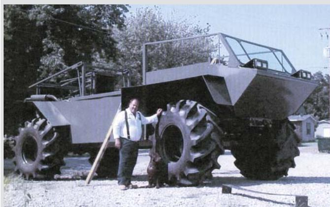
Kim Bickett turned his home-built amphibious tractor end-for-end, repowering it with a bigger engine and also adding a water propeller.
