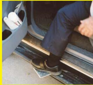
A local man in his 70's came up with this simple running board-mounted "swivel step", which makes it easier and safer to get into a pickup cab. Made from diamond plate steel, the step measures 4 by 6 in. It swivels inward, when not in use, on a nutted bolt that extends through the step and into a hole drilled into the running board. **(Rex Gogerty, 33475 K. Ave., Hubbard, Iowa 50122, ph 641 487-7617)**
