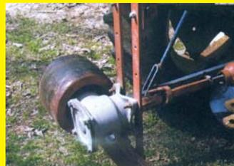
After you ran the article on my pto-powered belt pulley in your last issue, I got a letter from Wayne Beggs, Lincolnton, Georgia, with a picture of a Ford belt pulley. He had a 3-pt. mount for his tractor, and uses a short pto shaft to connect to the input side of the pulley. He set this up 20 years ago to power an old gristmill. **(Warren Farley, Jackson, Ohio)**
