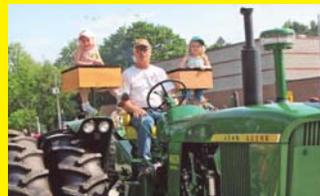
the tractor fenders. Each seat sets on top of a telescoping metal pipe, so by pulling a pin I can adjust the seat up or down and also rotate it. When I use the tractor for field work I remove the seats from metal brackets bolted onto the fenders.
