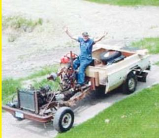
old Chevy 4-WD pickup and a Deere front-end loader. It has an automatic transmission, power steering, and power brakes, which is a big improvement from the Oliver tractor he was driving before. It's much easier for him to steer now that he's 72 years old. **(Connie Frederick, Troy, Mont., ph 406 295-9277)**
