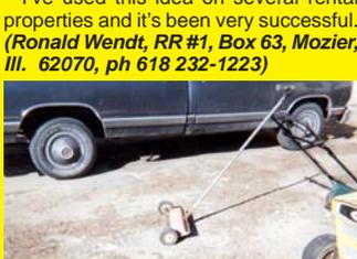
I mounted wheels and a handle on a magnet that came off an old Letz feed grinder. It's a very strong magnet and works great to pick up nails and other metal parts. **(Floyd Woznick, Bridgeport, Neb.)**
