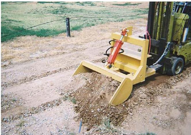
Mini dump bucket hooks up with adapters that slip onto forklift forks. It can be powered by forklift hydraulics or electric hydraulic pump.
