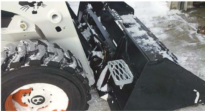
Handy step for Bobcat skid loaders bolts to back of bucket, making it easier to enter and exit cab.
