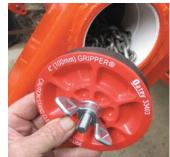
Dan Bodas stores chains, tools and pins in 4-in. dia. tubes on his Kubota tractor loader, covering the ends of the tubes with 4-in. dia. pvc expander plugs
