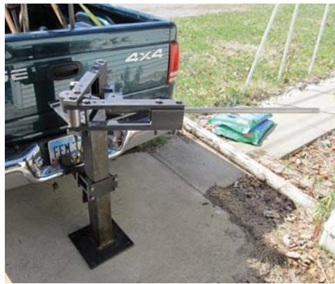
**Portable metal bender fits into receiver hitch on back of Warren Farley's pickup. "It'll bend steel up to 3 in. wide and 3/8 in. thick," says Farley.**
