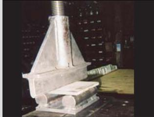
"I use several different bottom dies with our hydraulic press. The one shown in the photo is made from 1 3/4-in. dia., 6-in. long rounds set 4 in. apart on a 1/2-in. thick steel plate. My 50-ton press can bend 1/2 by 6-in. bars on it.
