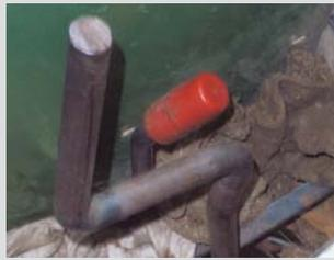
"The pto control lever on my Deere 5000 series tractor broke off in my hand one day when I was using it, so I decided to replace it with one that I made out of 3/4-in. dia. solid cold-rolled rod. I heated the tubing and made a double bend handle at the top. The handle extends much farther off the operator's platform than the factory one, so now I don't have to reach as far to engage or disengage the pto. And, there's enough room underneath the handle for my chainsaw."
