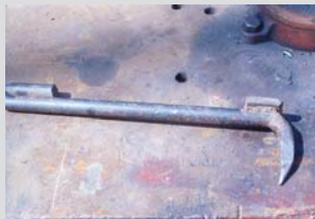
works great for removing deeply embedded staples from trees and posts. The tool has good balance and feel, and there's a piece of strap metal welded on top to hammer on.
