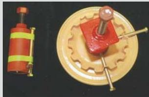
**Leonard Hodges, Callaway, Va.:** "The starter pulley on Cub Cadet garden tractors can be easily damaged when you try to remove it because it's made from lightweight metal. A new replacement pulley costs about \$35. To solve the problem, I made a puller that prevents the damage. I have a few in stock, and they sell for \$50 plus S&H.
