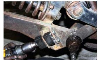
**Repair involves drilling out the hole on seed boot mounting lug, then installing a hardened full length bushing.**
