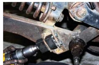
**Repair involves drilling out the hole on seed boot mounting lug, then installing a hardened full length bushing.**
