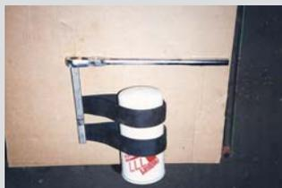
**Roger Avram, Twining, Mich.:** "I welded 2 oil filter wrenches together to come up with this dual strap oil filter wrench, which makes removing hard-to-turn oil filters a much easier job. The dual strap applies the load to a greater area which increases the torque, and it won't crush the filter like a single strap filter might."
