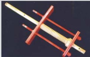
"I came up with a tool for my Cub Cadet garden tractor that compresses the spring on the tractor's driveshaft, making it easier to replace the tractor's throw-out bearing. It's a safe way to get the job done. Anyone who's interested can call me and I'll tell them how to make it."
