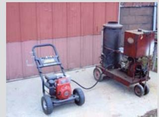
good shape. I plumbed in a 4-ft. hydraulic hose from the tank from the heater to the washer. Now I have 3,000 psi of hot water (approximately 150°) all for a few dollars. Works great to clean grease off equipment."
