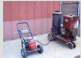
good shape. I plumbed in a 4-ft. hydraulic hose from the tank from the heater to the washer. Now I have 3,000 psi of hot water (approximately 150°) all for a few dollars. Works great to clean grease off equipment."
