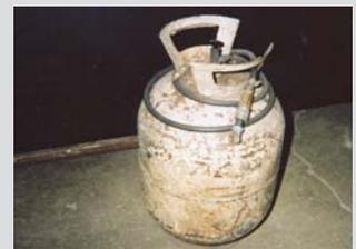
coupler that's used to fill the tank with air. Then he screwed two male coupler ends together to fill it from a supply air hose. Works great for airing up low tires in the field or operating small air tools.
